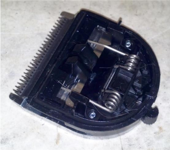
The “Open” version is the most common of the variations. It has an “spring deck” that is not covered and can hold hair. This version needs to be cleaned often of hair. The spring that holds the cutter down is strong and is “locked” into the plastic spring deck and shouldn’t move during use.
