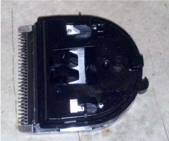
The “covered” version of the 5-N-1 blade was designed to keep hair from getting into the spring deck, and affecting the way the blade cuts. If hair does get inside, its very hard to clean it out. We have opened these blades during the refurbish program and hair was impacted inside this cover. These blades cost more than the “open” version.
