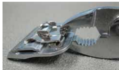
Bending the socket until it is parallel with the bottom of the blade.
