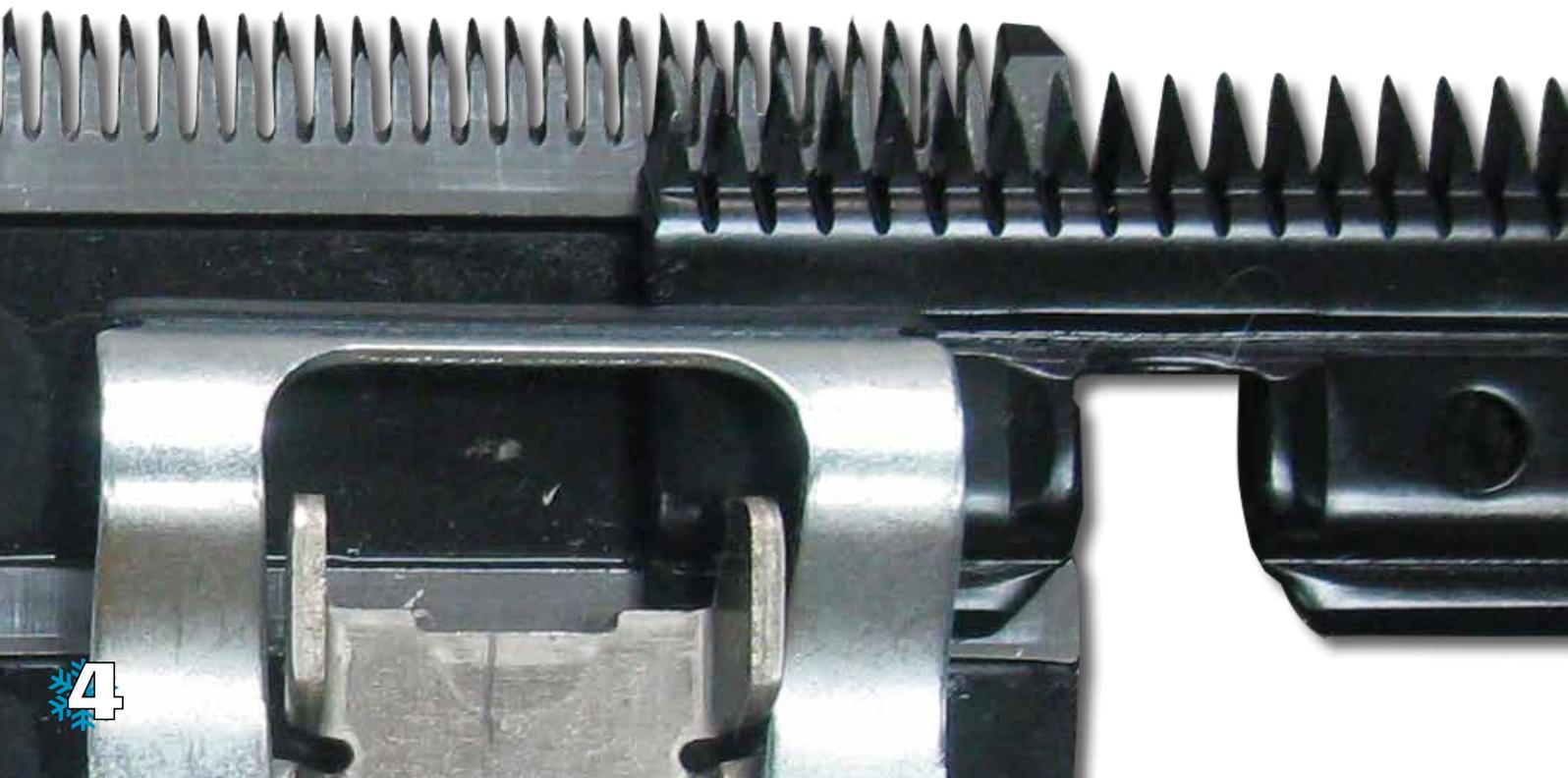
To clean the blade, slide the cutter to one side. Then, use a small brush (or toothbrush) to clean the cutter, comb, and spring of all hair, oil, and dander. Once the first side is clean, slide the cutter to the opposite side and repeat. Do not take the blades apart to clean them.
