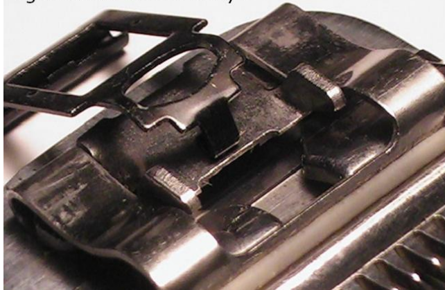
Latch hook not locked on socket and pushing against the socket body.
