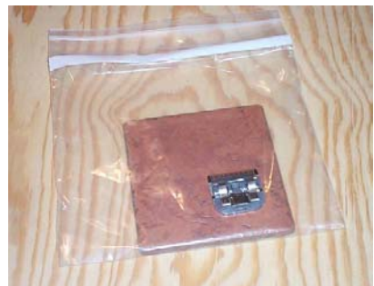
Frozen ceramic tile inside a plastic bag cooling blade
