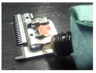
To start, put one tiny drop of oil on both rear rails. The first on the rear rail just outside the left spring as shown, and the other tiny drop on the rear rail outside the right spring where sliding the cutter over has given you access.
