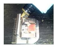
The third tiny drop goes in the grove in the top of the cutter. If you don't oil this grove at least once a day, your blade can have a screeching sound and not cut properly. Without oil, a dry blade guide will make the cutter hesitate. It may cause the blade to cornrow and other problems.
