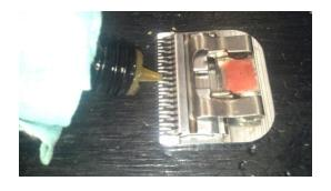
While on the table, or preferably on the clipper, put one tiny drop of oil in the center of the blade on the cutting surface. DO NOT RUN A BEAD OF OIL ACROSS THE TEETH, IT WILL SEEP DOWN THROUGH THE TEETH AND GET ON THE COAT. Start the clipper up, the oil will spread a thin coating across the blade. That's all you need.
