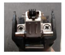
If you use combs a lot, especially on an Andis clipper, the hinge screws can loosen. This is because of the pull and vibration of the comb through coat. The screws loosen because they are screwed into plastic threads in the clipper housing, not metal. These screws should be checked weekly, and if they turn even a tiny bit could mean a lot of looseness in the system. You may see cornrows in the coat with or without a comb. Hair can jam on the comb also.
