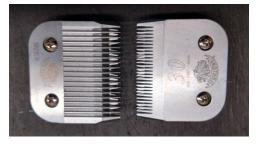
Suggestion: When you get a new blade, or a blade back from the sharpener do this. Try the blade on the dog someplace (belly) before putting the comb on it. If it cuts hair without a comb, and doesn't with the comb, the problem isn't the blade. You need to start looking for something that's loose in your system.
