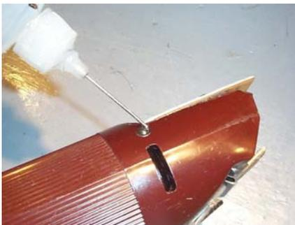
*Finally, take clipper oil and lube the armature gear. It only takes a drop but its very important to do this.*
