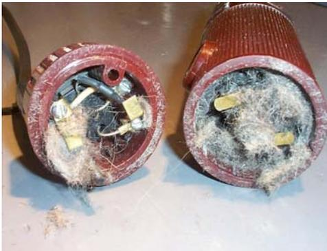
*Taking the rear switch housing off and checking for compacted hair is another routine maintenance item. Not blowing this out routinely blocks the airflow to the armature and will burn it up. You will also notice the unit getting very hot very quickly during use.*
