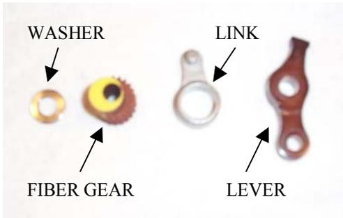
*With the gears all out, clean them thoroughly and check for damage. Look closely at the fiber gear and make sure there isn't a groove worn in the middle of it. Replace if the groove is real deep.*
