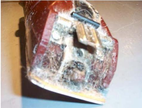
*The clipper head needs to be blown out with your hair dryer on a daily basis. Not doing so will clog the air flow and could prevent the blade from seating securely on the hinge and latch. A dirty latch could give "blade wobble" or a "corn rowing" effect on the cut. Hinges and latches don't last forever and may need replaced.*
