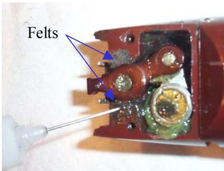
*Oil the felts with clipper oil. Not too much but enough to make them look dark. The felts will be gray in color if they are dry, and will cause the lever to overheat as it rocks back and forth. Oiling also gives a tight fit around the lever.*
