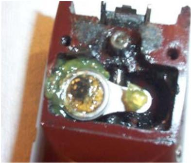
*Replace the link. Make sure there is grease on the top of the fiber gear so the link will slide easy.*
