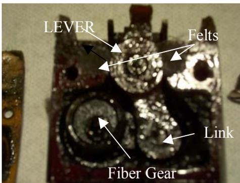
*Take the gearbox plate off and expose the gearbox. Take a set of needle nose pliers and take all the gears out. Pull the lever out, then the link, then the fiber gear and washer. **DO NOT REMOVE THE FELTS ON EACH SIDE OF THE LEVER.** Then take Q-Tips or paper towel and get as much of the dirty grease out of the gearbox.*
