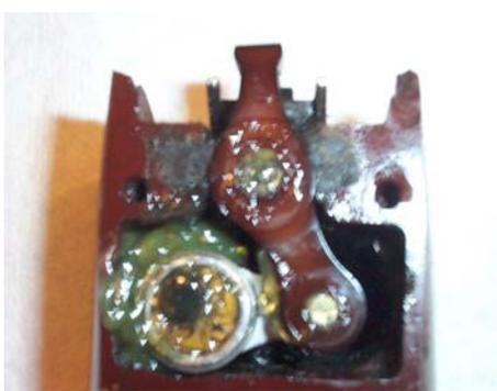
*Before installing the lever put a small drop of grease in the center hole. Do not grease the post where the lever attaches you might get grease on the felts.*
