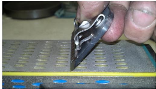
Run the blade back and forth with a slight downward force to let the diamond do its work (a motion like buttering your bread). Go back and forth a few times and check it with your finger. Do it until you feel its safe to use.
