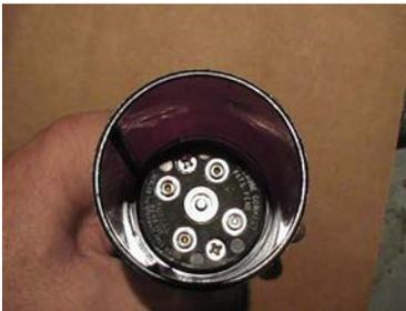
Now look down inside your clipper housing where the cordpack or battery fits into. There are four "male" connectors that almost look like the same part of the "snap". The problem we have is that over time as these connectors have come together countless times, the male part has spread apart the sides of the female part. Now, it doesn't want to snap together and hold like it did when it was new.
