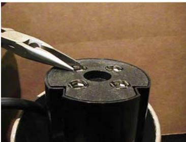
To fix this problems, grab your needle nose pliers. With your pliers, gently squeeze the sides of the female connector so they move just a very little bit There's not much of the connector sticking above the surface of the face-plate, but you can still bend them slightly. Don't bend them in too far or you'll have t bend them outward again. This will tighten this connector so it will "snap" on the male connector, keeping the cordpack or battery from falling out anymore. Good Job!
