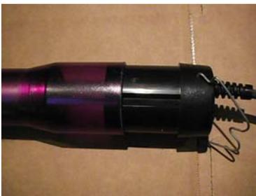
If you've done it correctly, you should be able to re-insert your cordpack or battery and it will snap into the other connector securely. You may have to push it hard the first time to snap it.
